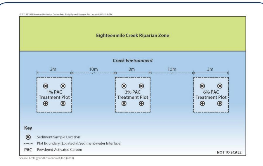
Figure 1 Example Plot Layout for Powdered Activated Carbon Field Study (Plan View)
