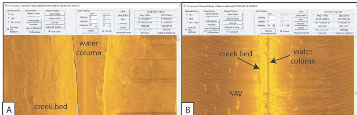
Figure 2: Example of water column identification in the sidescan data for regions both with and without SAV. (A) Region with no SAV and software-defined sediment/water interface. (B) Region with SAV growth obscuring the creek bed and a user-defined sediment/water interface.
